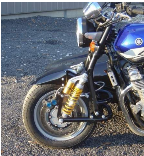
Fairly typical leading link forks. Susceptible to tyre 'lift' and 'flex', but good for steering lock. Photo: DJ Construction © 2017
