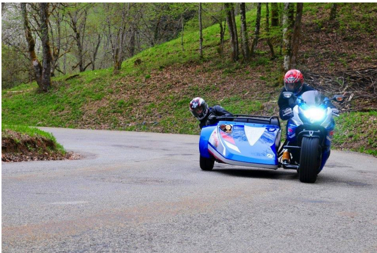
Suzuki GSX and DJ Sport Sidecar. Notice width of chair facilitates weight transfer and the twin 'wishbones' by the front wheel. Photo: DJ Construction © 2017
