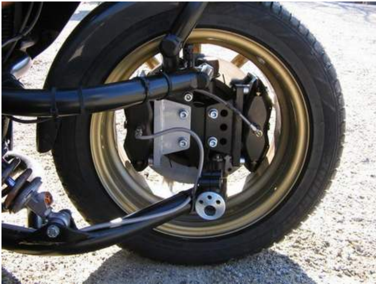
DJ's Hub-Centric layout. Much less prone to 'lift & flex', but wishbones can restrict lock on one side. DJ Construction © 2017
